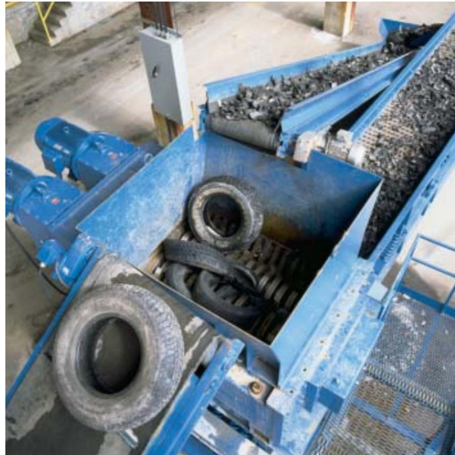
**ST 150E Tire Shredding System Reduces Automobile and Truck tires to a 2" minus chip size @ a rate of 6TPH**
