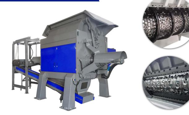
This high-powered single shaft shredder with a 620 mm rotor, hydraulic drive and low rpm can be equipped with a radial pusher or drawer pusher depending on the material being processed.
